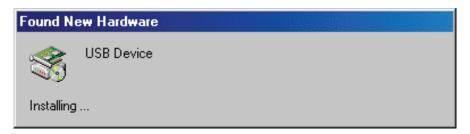
Go on following the wizard, and a dialog box for specifying the setup information file (inf file) is displayed. Specify the musbdrv.inf file stored in a location below the directory where this debugger is installed.
